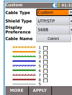
Use a list of wiremap templates for common Ethernet cable types as well as non-Ethernet cables, such as Profinet and ISDN.
