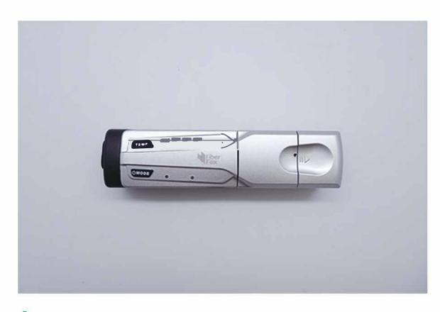
1. Turn on the heating stripper and set the right mode and temperature.
