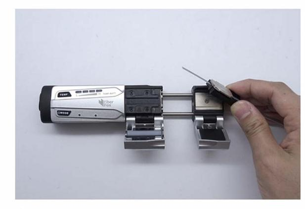
2. Open the both covers and put the holder with fiber on the right slide.
